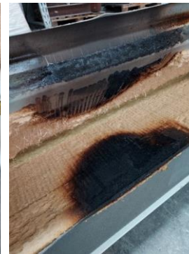
c) Flat roofing sandwich panel with insulation and waterproof membrane
