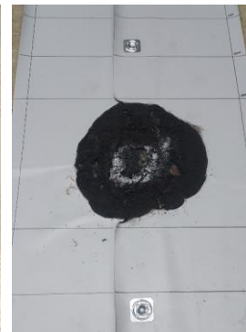
c) Flat roofing sandwich panel with insulation and waterproof membrane
