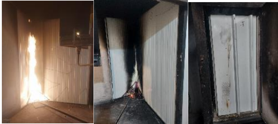
Figure 4. SBI tests of roof sandwich panel systems during and after the tests
