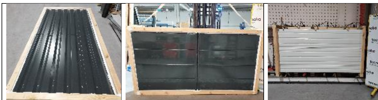
Figure 3. The double skin system and façade cladding with cassettes before and during the air permeability test.
