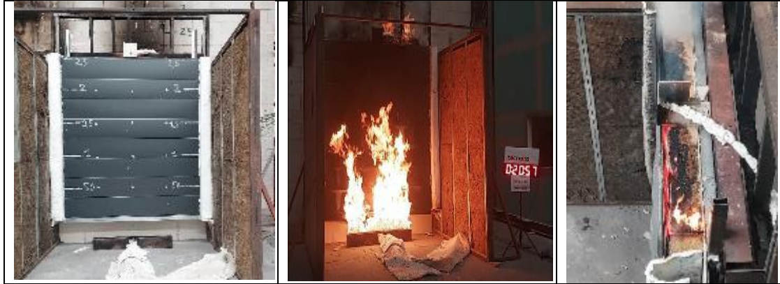
Figure 5. Cassette cladding system before, during and after the fire propagation test.
