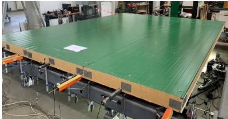
Figure 1 Cladding panel and its fixing under diaphragm testing
