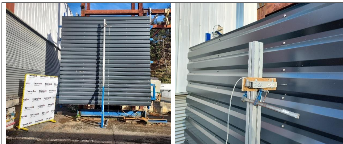
Figure 2 Double skin cladding system during the seismic tests
